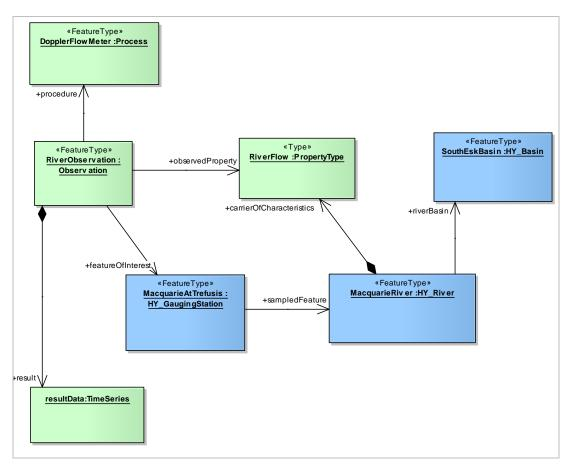
Figure 8 - Example river flow observation in UML
